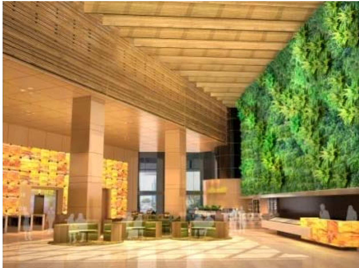
After AEI – the “green” wall reduces indoor heat gain and the onyx reused at other parts of the lobby
